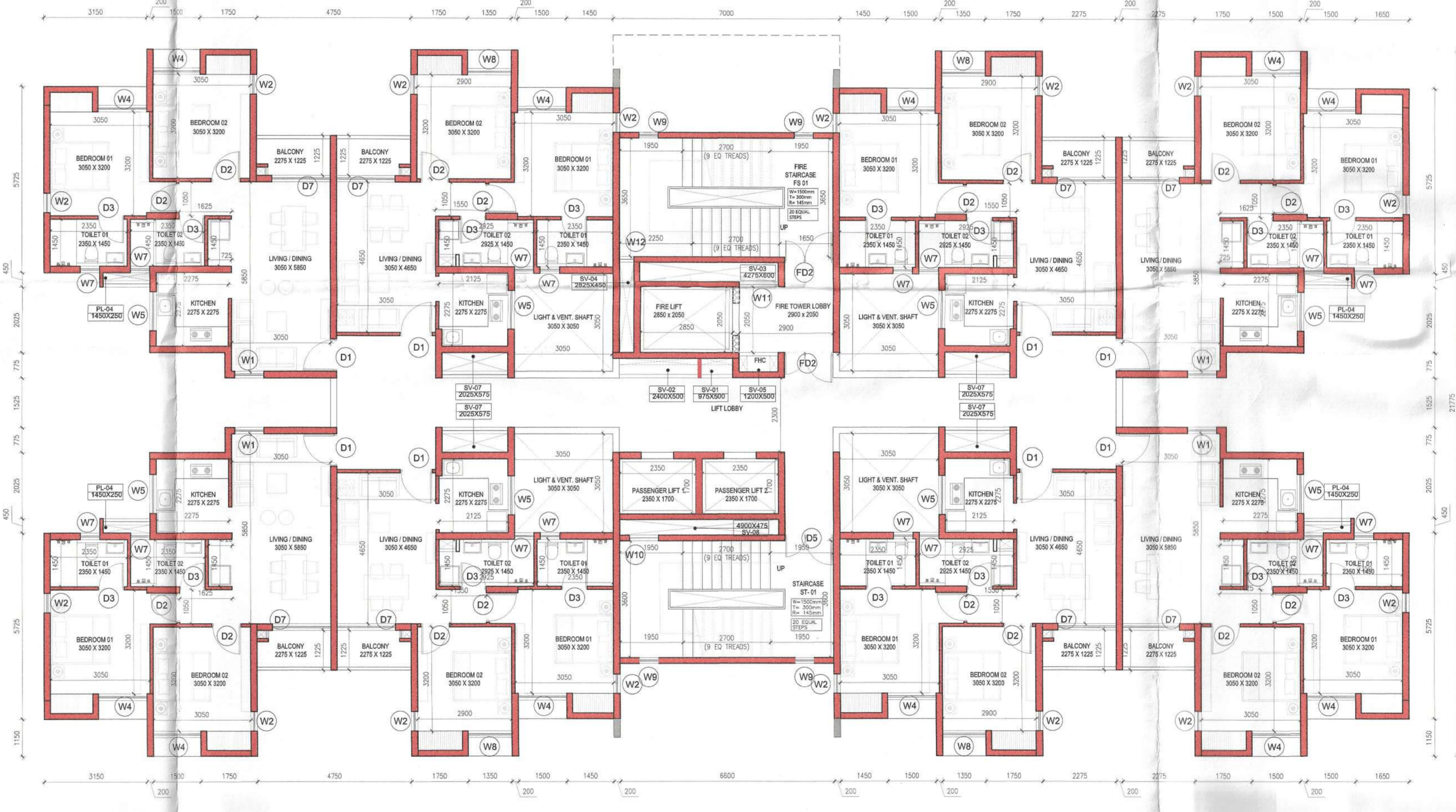
4 TOWER C1 TYPICAL FLOOR PLAN (3rd to 7th, 9th to 12th, 14th to 17th and 19th) 1:100
